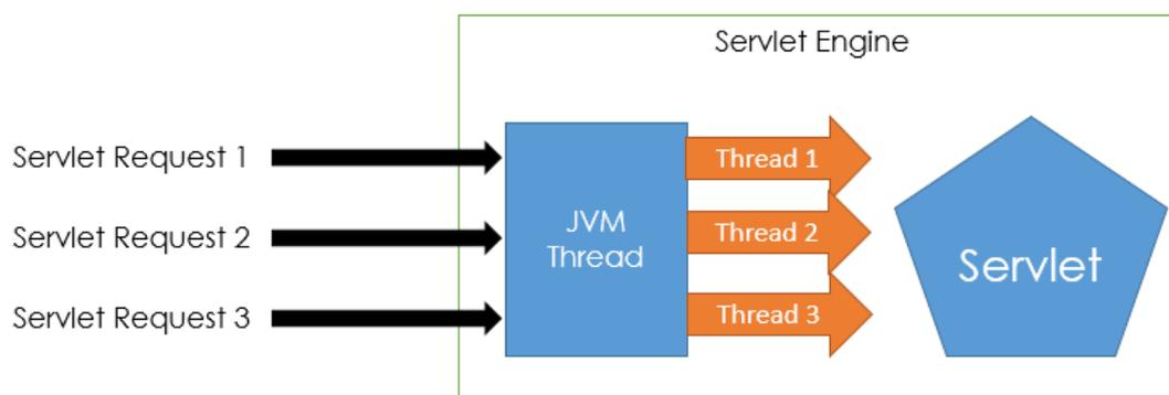
In Servlet, All the requests coming from the Client are processed with the threads instead of the OS process.
