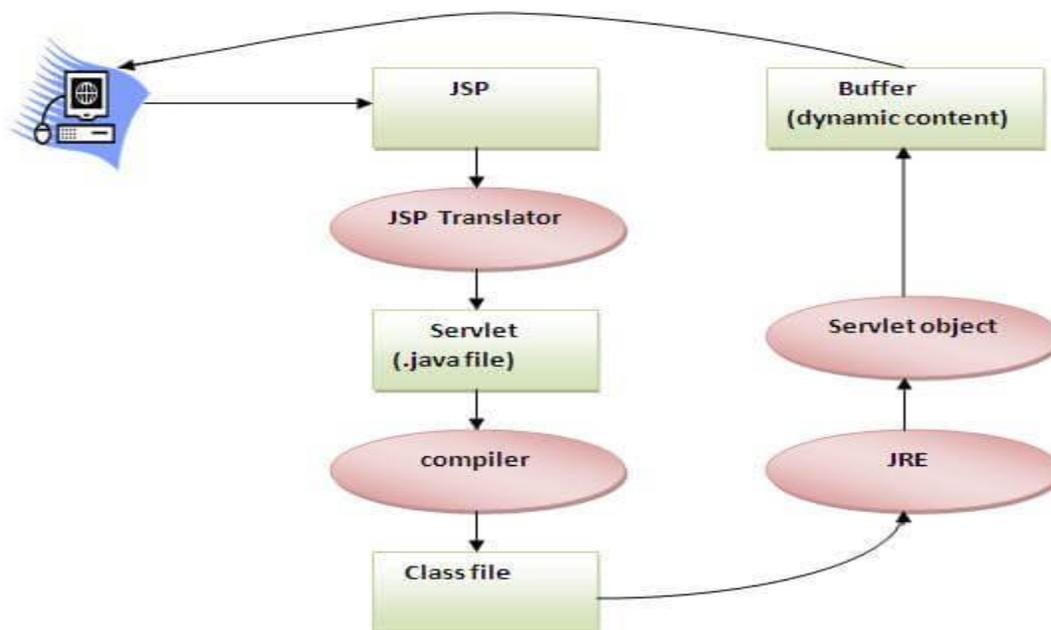
As depicted in the above diagram, JSP page is translated into Servlet by the help of JSP translator. The JSP translator is a part of the web server which is responsible for translating the JSP page into Servlet. After that, Servlet page is compiled by the compiler and gets converted into the class file. Moreover, all the processes that happen in Servlet are performed on JSP later like initialization, committing response to the browser and destroy
