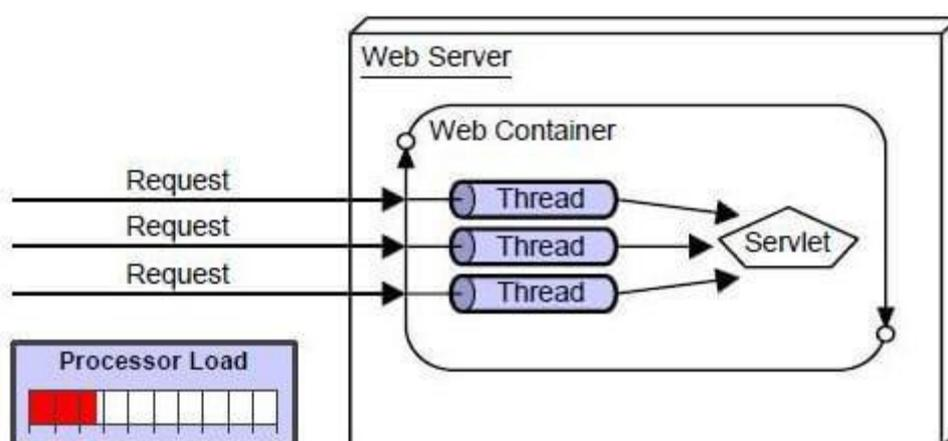
There are many advantages of Servlet over CGI. The web container creates threads for handling the multiple requests to the Servlet. Threads have many benefits over the Processes such as they share a common memory area, lightweight, cost of communication between the threads are low. The advantages of Servlet are as follows:
